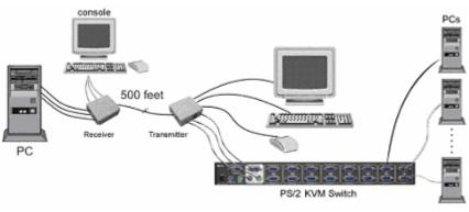
Figure 2-3: Connecting to a KVM
